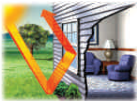
In summer months, Low-E glass filters the sun's rays and reduces heat penetration from solar energy.
