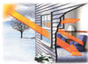
In winter months, Low-E glass lets warm solar rays into your home, while preventing indoor heat from escaping.
