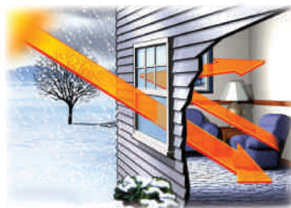
Low-E glass takes on a new duty in winter months. It lets warm solar rays into your home, while preventing indoor heat from escaping.
